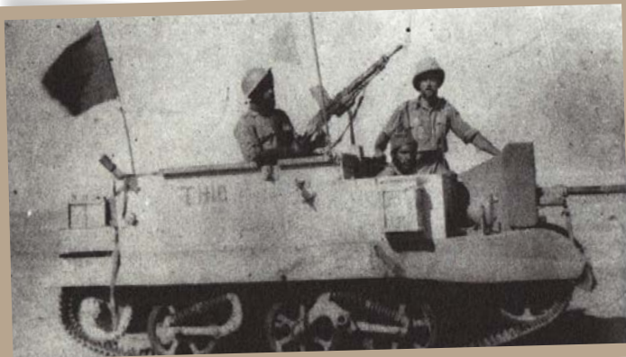
Modified Bren Carrier with 25mm AT gun
